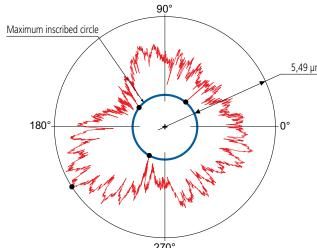
The position of the center of the concentric circles defines the center of the extracted circumferential line and therefore the location of the circular feature measured. Each of the methods described above results in different center positions for the reference circles, as shown below.
