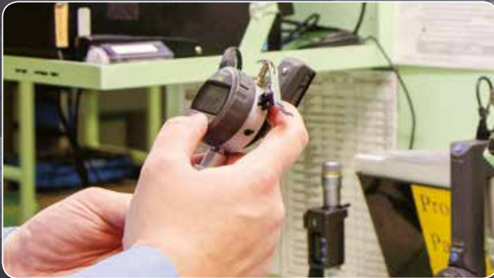
Inspection being performed at the point of manufacture. Sampling techniques based on capability reduce the time spent on inspection while still ensuring the quality of the product.
