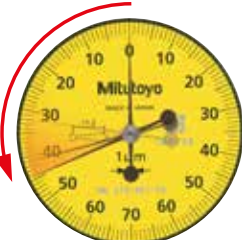
Indicator trackability depends on maintaining gear-train stability
