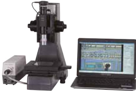
Digital microscopic system using VMU-V
