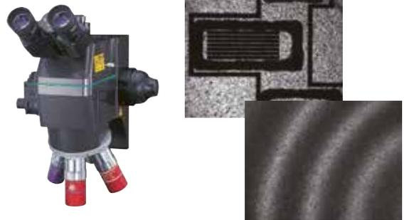
Optical systems using Mitutoyo M Plan Apo NIR objectives that cover a wide range of wavelength from visible to infrared are providing solutions on the production line and in the laboratory. Nondestructive inspection is made possible by using an infrared source.
