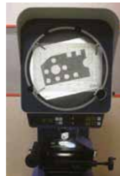
View comparison using the profile projector (drawing as a template)
