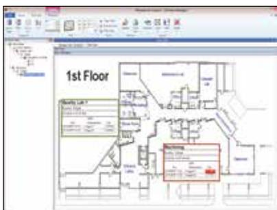
MeasurLink Process Manager displays snapshot windows of characteristics that are currently being collected in MeasurLink Real-Time. The data can be sorted by Station, Process, Capability or Timestamp.
