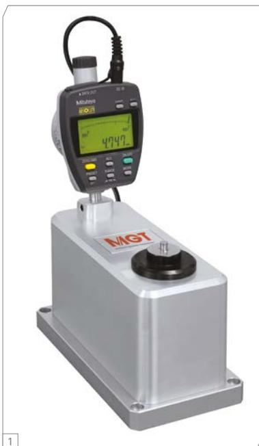
The performance of bench gauging instruments can be significantly enhanced by carefully thought out fixture design to enable application to a wide range of measurement types. MGT has designed and delivered countless examples of fixtures that enable these basic instruments to perform measurement tasks well beyond the traditional boundaries of use.
