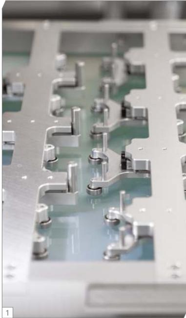
Although VMMs are usually regarded as 2D measuring machines, with the addition of carefully designed fixturing they can be extremely useful for inspecting 3D products. MGT has designed and built many VMM fixtures to enable measurement of roundform components that would otherwise require a different kind of measuring machine to be available.
