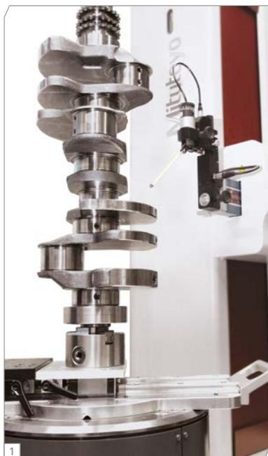
The scope for increasing the usefulness of these types of measuring machine is practically limitless. MGT makes a speciality of designing and building highly specialized fixtures that enhance versatility by incorporating standard accessories such as turntables, indexing heads, XY tables, centre supports and calibration artefacts.
