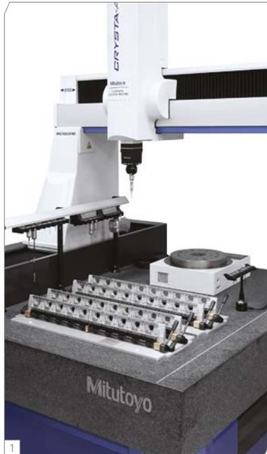
*In the case of the CMM, the extensive selection of probing systems available enable this general-purpose machine to tackle almost any measurement task without further assistance. However, there are situations that benefit from the use of custom fixtures to position and hold components to the best advantage for measurement.*
