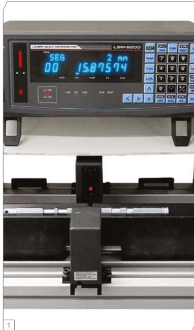
MGT has extensive experience of maximizing the performance of the laser micrometer with custom fixturing that takes advantage of the exceptional performance of the instrument in measuring diameters on roundform components. It is vital to ensure that the fixture centres the feature of interest repeatably within the measuring region for maximum accuracy, especially if this involves translation and/or rotation during the measurement cycle.
