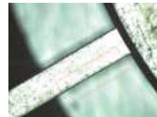
Positive edge detection with co-axial light
