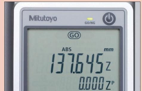
GO on the display and the panel LED showing GREEN means the measurement is within the tolerance limits.
