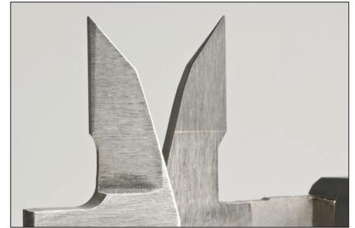
Carbide-tipped jaws for inside measurement.
