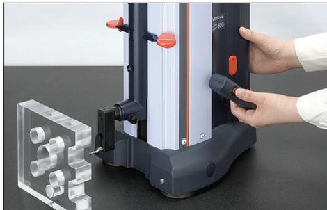
The power grip makes it easy to approach the workpiece.
