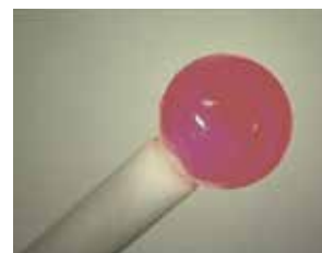
Cleaned stylus tip
