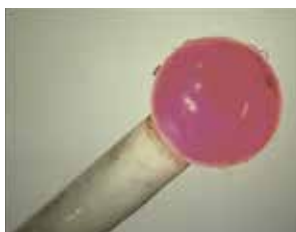
Contaminated stylus tip
