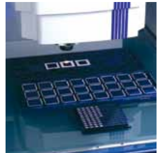
Measuring without workpiece clamping
