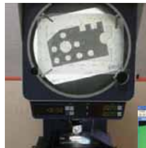
Comparison using a profile projector with engineering drawing as template
